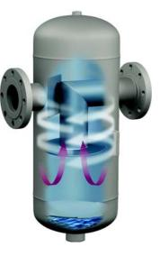
The complexity of the Type R is slightly more than the Type T due to the addition of a secondary vortex. Instead of the gas exiting through the low velocity
